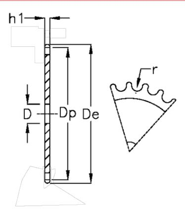
C = 1 D = 12 De = 110.4 Dp = 106.26 For chain size = 3/8 x 7/32 For chain type = 06 B-1 h1 = 5.3 Solution Number of teeth = 35
